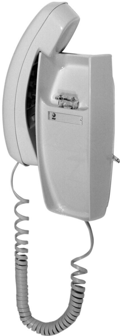
Fig. 48. Trimline off-hook handset on revised wall-mounted base, ca. 1968. (Ralph Meyer.)
