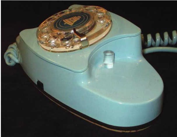
Fig. 34. Field-trial Princess showing two-piece construction, 1957. (Paul Fassbender.)
