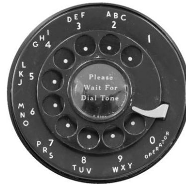
Fig. 24. Western Electric dial for 500 showing white dots, 1949. (Ralph Meyer.)
