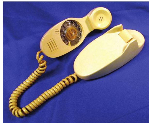
Fig. 37. Western Electric dial-in-handset (Shmoo) telephone, 1959. (Paul Fassbender.)
